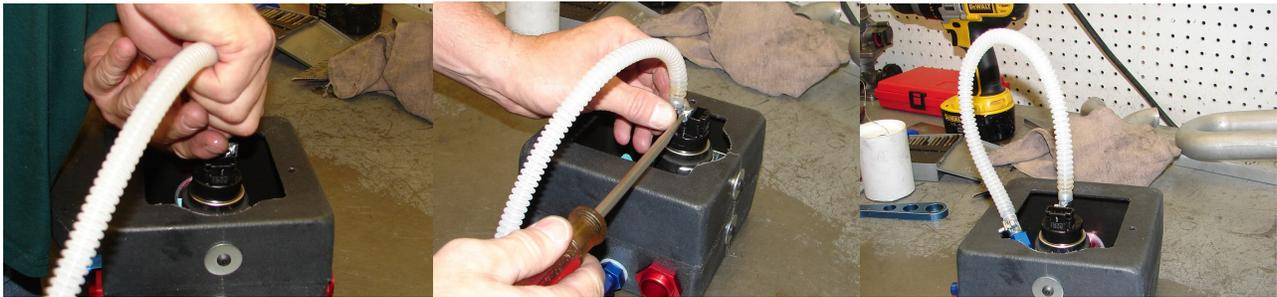
7. The electrical bulk head fitting should be located as high as possible on service plate. So it's not constantly in liquid fuel.
