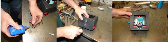
Set the box on the bench and make sure the pump is resting on the floor of the surge box and tighten the wire tie's. You can bend the filter sock and let it lay on the check valve body or place it under the check valve body directly across from the pump.
