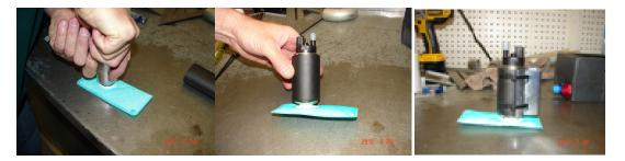
Now lay the pump on the bracket and wrap the wire tie's around the pump and through the holes in the bracket. Leave them loose.
