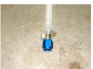
Add the second clamp to the other end of the hose. With the same procedure, surge box sitting on the bench push the hose on the pump nipple. Tighten the clamp in the middle of the straight area of the nipple
