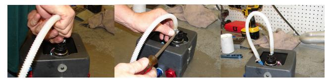
7. The electrical bulk head fitting should be located as high as possible on service plate. So it's not constantly in liquid fuel.
